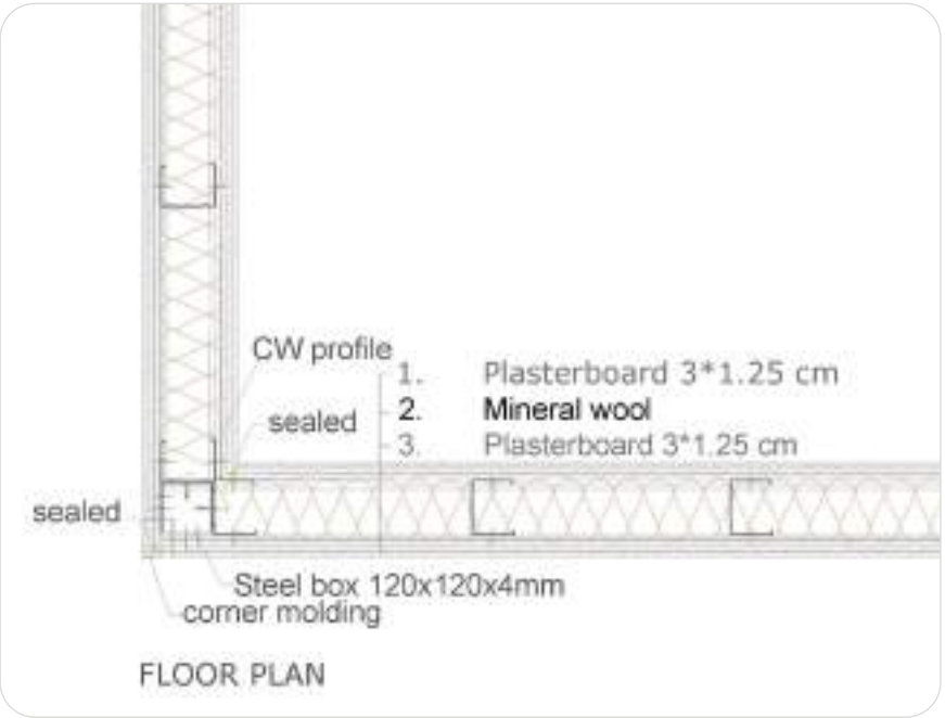
Figure 4.3.2.7 — Pavilion Façade_detail 3
